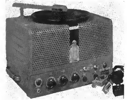
RCA SOUND SYSTEM for use in mobile, portable, or permanent installations. Operates from 105-125 volt, 60 cycle power or from a 6 volt battery. Delivers 15 watt output and is available with or without the turntable and pick-up. Measures 16½ long, 12 deep, and 12 inches high. RCA Mfg. Co., Camden, N. J.
